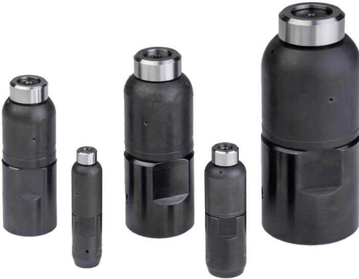
The DrillJet™ is a self-powered rotating nozzle designed for tube cleaning available in five sizes with a variety of inlet options. The DrillJet™ is a universal type of tool with six or seven nozzles that clear blockages, clean, and provide thrust to propel the tool down the pipe. The tool is available in a range of pressures and flows depending on size.
